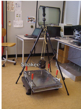
Figure 7.10: Setup of the shaker test.
