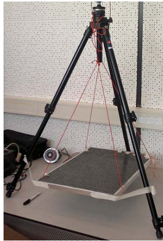
Figure 7.9: Setup of the impact hammer modal test.
